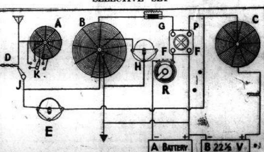
Hook-up Diagram of Improved Reinartz Circuit
