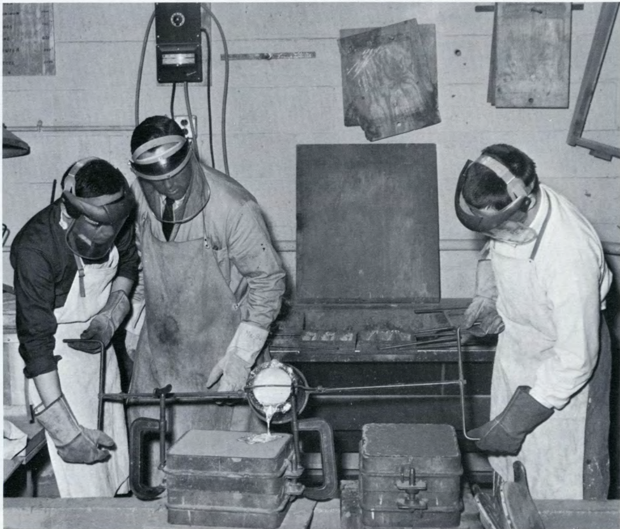
Mr. Sullivan directs the pouring of a mold.
