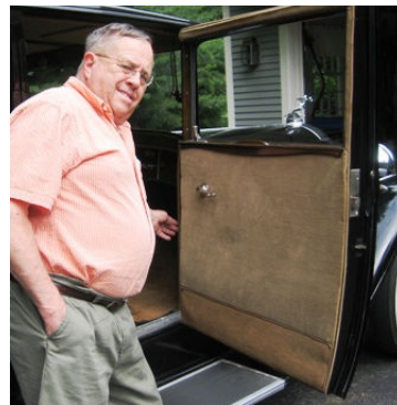
Marshall shows the “windlace” inside the Packard’s door. Due to its location, this long upholstered piece would ordinarily get a lot of wear and tear, but it’s in original condition thanks to Mary O’Leary’s care.
